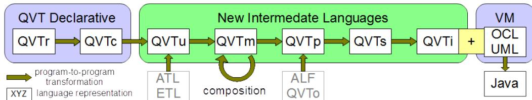
The Eclipse QVTd support involves a transformation chain from QVTr via QVTc to executable form. The stages in this chain are:
